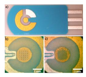
FIG. 1. (Color online) (a) A picture of a gold SPE (Dropsens C223AT) sensor. (b) Discrete thylakoid pixels printed by LIFT on the working electrode of the SPE sensor. (c) A continuous thylakoid layer printed by LIFT on the working electrode of the SPE sensor.
