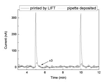
FIG. 2. For comparison, typical electrical signals for printed by LIFT (black line) and pipette deposited (gray line) sensors.
