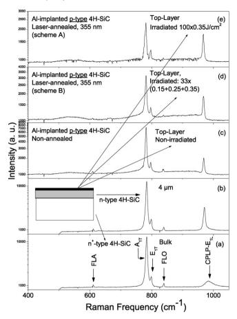
Fig. 2. Cross-sectional micro-Raman backscattering spectra from different regions of the as-implanted sample as well as the top layer of various irradiated samples.
