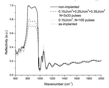
Fig. 1. Infrared reflectivity spectra of non-implanted, as-implanted and laser annealed 4H–SiC samples at 355 nm.
