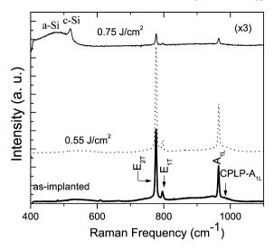
Fig. 3. Characteristic front-view backscattering micro-Raman spectra of asimplanted and laser-annealed samples. Spectra are shifted for clarity.
