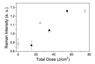
Fig. 4. The integrated intensity of the transverse optical  $E_{2T}$  (776 cm<sup>-1</sup>) mode, as a function of the total energy dose of the annealing laser beam at 355 nm, for (a) a sequence of samples irradiated with 100 pulses and energy density per pulse, 0.15, 0.35 and 0.55 J/cm<sup>2</sup> (solid squares) and (b) a sequence of samples treated by the 'multiple irradiation method' at 0.15, 0.25 and 0.35 J/cm<sup>2</sup> with either 33 or 100 pulses at each energy (open circles).
