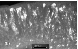
Fig. 5. (a) Bright field and (b) dark field cross-sectional TEM images of the laser annealed 4H-SiC/Al implanted under the multiple irradiation method.
