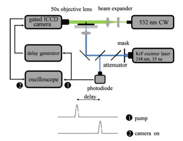
**Fig. 1.** A sketch of the shadowgraphic time-resolved imaging setup. A pump KrF eximer laser (248 nm, 35 ns) initiates the ejection of silver NP ink. The images are captured with a gated ICCD camera, which is synchronized to the pump laser through a photodiode and a pulse delay generator. Both photodiode and ICCD signals were sent to an oscilloscope for accurate measuring of the delay time.
