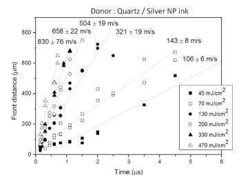
**Fig. 5.** LIFT of silver NP ink without using DRL. Plot of the front material position as a function of the time delay with respect to the pump laser pulse. The standard error of the slope was used to determine the corresponding standard error for the velocity.
