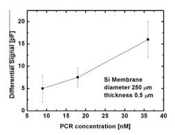
**Fig. 4.** Average response of the CD19N functionalized sensors, in respect to the mutated, to 36, 18 and 9 nM PCR concentration.
