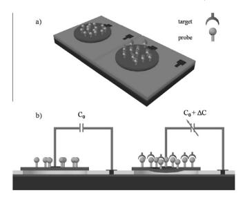
**Fig. 1.** Schematic of the capacitive sensing element: (a) top view, (b) cross section view.
