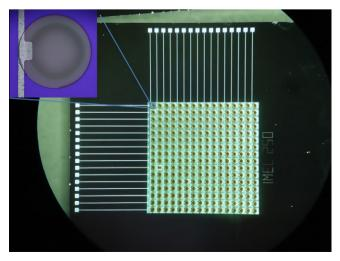
Fig. 2. Fabricated biosensor array. In the inlet a biosensing element is presented.
