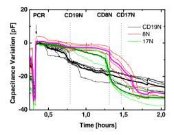
**Fig. 5.** Response of individual sensors and average response (thick lines) for 36 nM PCR. Three different oligos (CD19N, CD17N and CD8N) are depicted.
