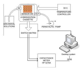
**Fig. 3.** Experimental setup. In a typical experiment the following solutions are inserted in the hybridization chamber: (1) tetramethylammonium chloride buffer (TMAC); (2)  $ddH_2O$ ; (3) the PCR product of the complementary strands, which remains into the chamber for several hours; and (4) TMAC in order to wash away the nonspecifically bound molecules.
