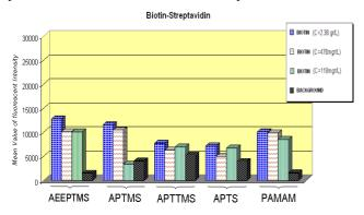
**Figure 2** Fluorescent intensity for the biotin-NHS - strepta-vidin-R-phycoerythrin (5 mg/L) reaction for five different aminosilane coatings of the LTO/Si surface.
