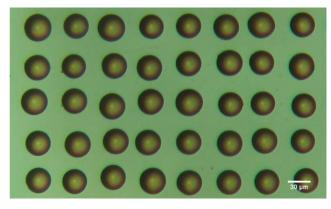
**Figure 3** Optical microscopy image of a biotin microarray on a silane coated LTO/Si substrate ( $\Phi = 260 \text{ mJ/cm}^2$ , 20  $\mu$ m spot size).
