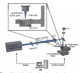
Figure 1 Laser induced forward transfer experimental setup.
