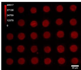
**Figure 5** Fluorescence microscopy image of the transferred droplets ( $\Phi = 120 \text{ mJ/cm}^2$ , 30  $\mu m$  spot size) obtained after the biotin-streptavidin reaction on a silane coated LTO/Si substrate.
