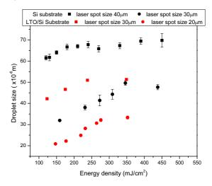
**Figure 4** Plot of the diameter of the transferred droplets versus the laser energy density for different laser spot sizes and substrates.
